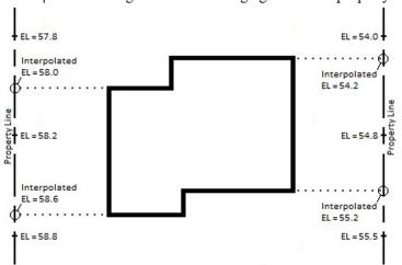
A property survey with elevations along the property line must be obtained, and the design professional must interpolate these elevations to determine the elevations adjacent to the building corners. The elevations must then be averaged on each side.
